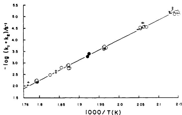
Figure 1. Arrhenius plot of the unimolecular rate constants  $k_{\text{tot}} = k_1 + k_2$  for the pyrolysis of 2,2-dimethyl-3-ethoxycyclobutan-1-one in the gas phase. The reaction vessels used are indicated with open circles (glass), closed circles (packed glass vessel), and plus signs (Teflon-coated reactor). Numbers indicate overlapping points.
